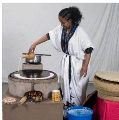
Figure 2 Cook Pouring Injera Batter on MIRT Stove
