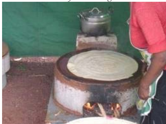
Figure 1 MIRT Stove with Injera Cooking
