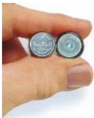
Figure 3 Electronic Stove Use Monitor
