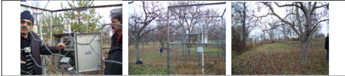
Figure 1. Weather stations are sited so as to monitor the microclimate of a typical orchard; as such, their siting does not correspond to WMO guidelines that would govern Turkey's basic weather monitoring network. The stations measure temperature, precipitation, wind, soil moisture, and leaf wetness, a different set of parameters from those measured at a basic weather station. PDA's current program does not draw on all these parameters, but further services to agriculture are possible and are envisioned
