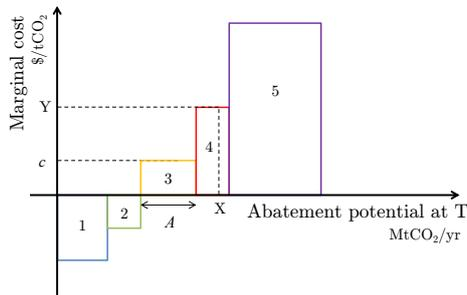
**Figure 1:** A measure-explicit marginal abatement cost curve. The general appearance of the curve suggests that it is meant to be used as an abatement supply curve, i.e. that the “abatement demand”  $X$  should be met by implementing measures 1 to 4, possibly using the carbon price  $Y$ .
