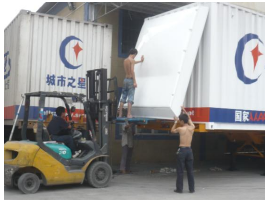
Figure 4: Nose cones of the brand DongGuan CAIJ installed on HDTs
