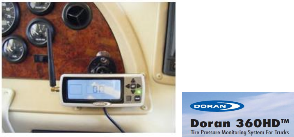
Figure 2: Tire pressure monitoring system
