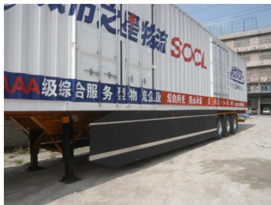
Figure 4: Nose cones of the brand DongGuan CAIJ installed on HDTs
