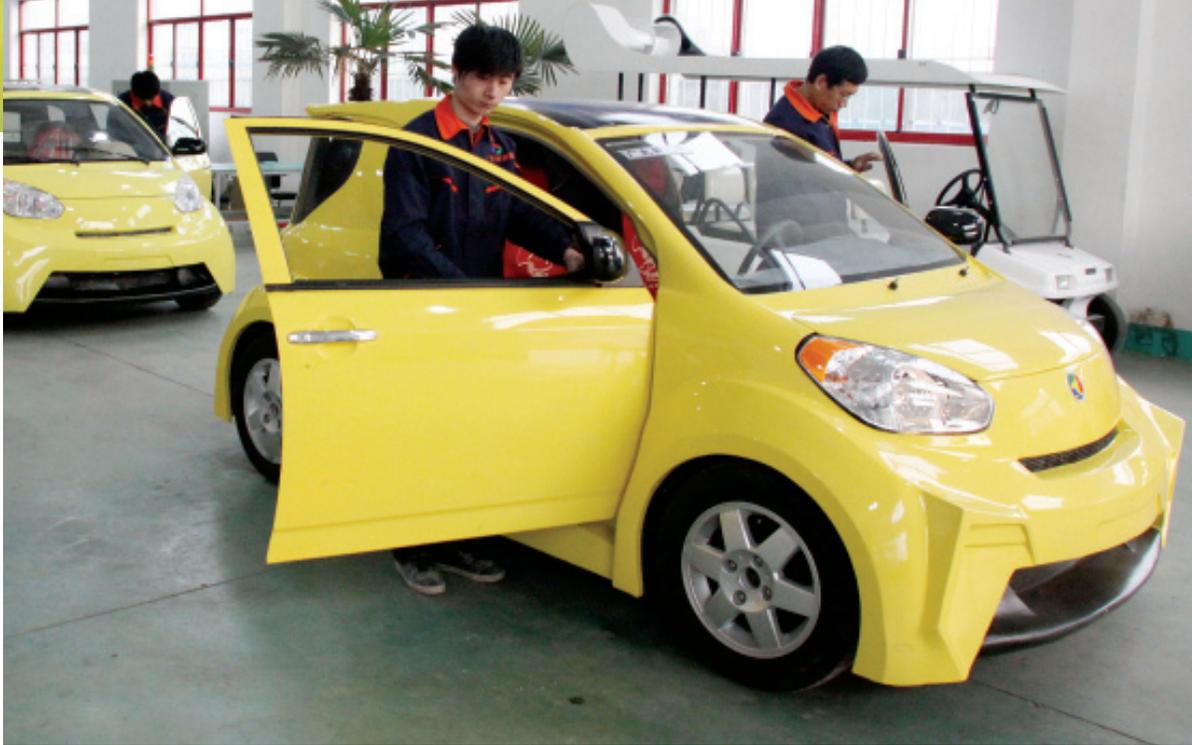
Workers assemble solar-powered vehicles in Weifang. Designed and manufactured by a Chinese company, the vehicle can run 120 to 150 kilometers under normal driving conditions on a full charge with speeds of up to 48 kilometers per hour. It has attracted its first batch of export orders from countries including Germany, the United States, and Norway.
