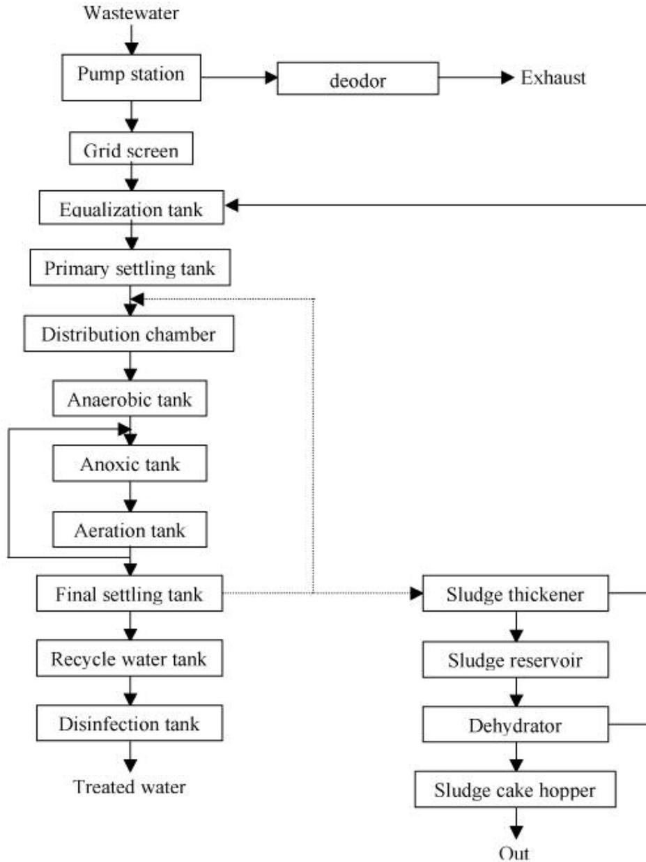
Figure 2: Process flow diagram of Truc Bach and Kim Lien WWTPs in Hanoi
