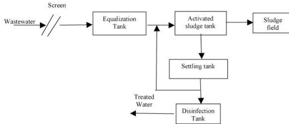
**Figure 3: Process flow diagram of typical wastewater treatment plant at an industrial zone**
