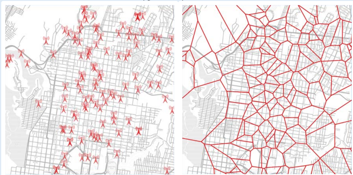
Figure 2: Sample Cell Towers around Guatemala City’s Constitution Plaza (L) and the Voronoi Polygons They Create (R)
